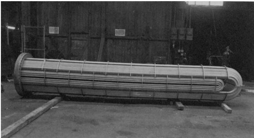
Photograph 14.c. Typical U-tube bundle.
