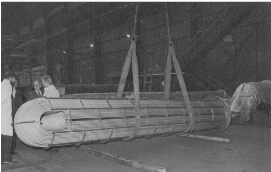
Photograph 22.e. Lifting a U-bundle using straps.
