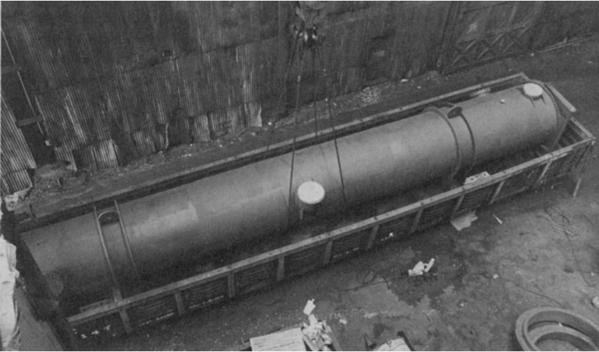
Photograph 12.a. Fixed tubesheet heat exchanger with hinge mounted flat cover (courtesy Joseph Oat Corporation).
